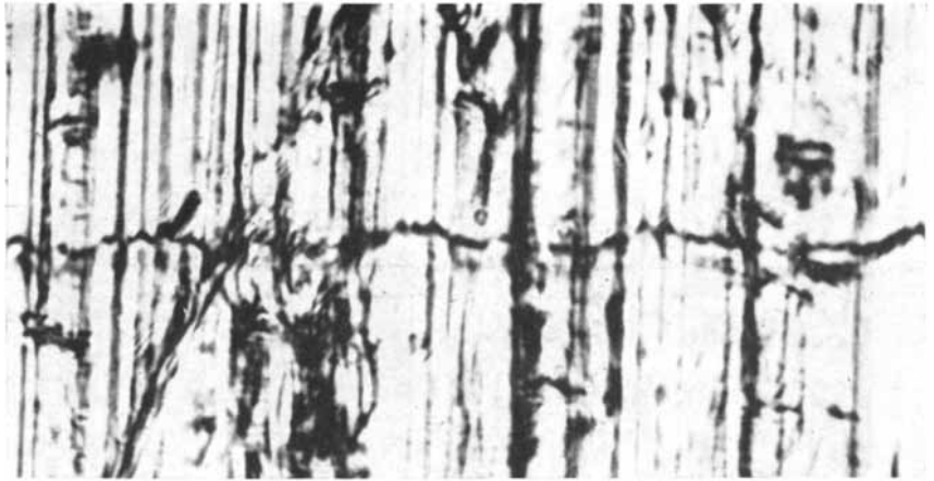
BEARING made on a boring machine was photographed by the light-profile method. The shadow line runs horizontally across the picture, indicating topography by its wiggles.
