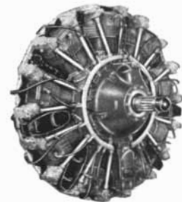
7- and 9-cylinder radial air-cooled engines.*
